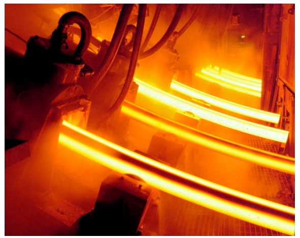
Steel exiting a continuous caster at a Tata Steel plant
